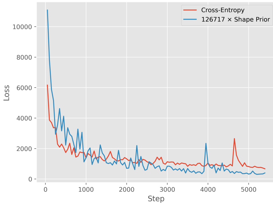
Figure B.1: Train loss graphs of U-Net trained with cross-entropy loss and ACU-Net trained with shape loss only ( \alpha = 0 ). The shape loss is scaled by \omega = 126717 to match the cross-entropy loss.
